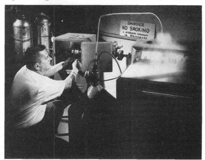
TEST SET-UP to measure permeation rate of hydrogen through silicone rubber is adjusted by J. P. Darginis of the Materials Application Division 8115. The rubber being tested is placed between two "hats" in small temperature chamber and hydrogen gas is passed through it into spectrometer (right) where permeation rate is computed. Liquid nitrogen, pumped into spectrometer from container (center) forms cold trap to obtain a test vacuum.
